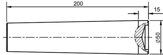
Part Name: Taper Pin Henred Fruehauf 200mm Drawing No: CC104.A or CC-0467 Weight: 3Kg
