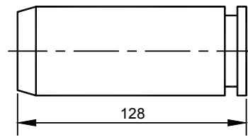
Part Name: Pivot Pin Drawing No: CC203 Note: Thomas Storey Removable Not currently in production – spares only.
